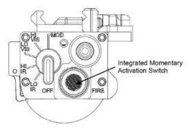
Figure 3-3 Integrated Momentary Activation Switch
