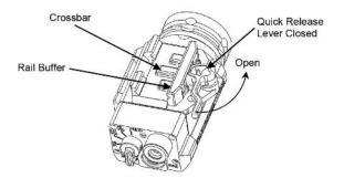
Figure 3-6 Quick Release Mount Configuration
