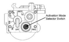
Figure 3-2 Activation Mode Selector Switch
