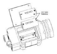
Figure 4-1 Battery Removal and Installation
